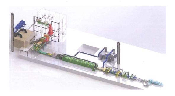
Production line type: Rock wool production line Width of production line: 1200 mm
